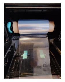
3. Install the roll of film on the under the print head, with the square end inserted in the wheel and the film lead from under the roll.
